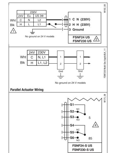
Auxiliary switch wiring for FSNF24-S US, FSNF230-S US
